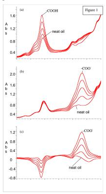
spectral contributions ratio out. The net spectral change observed is only what has changed as a result of the reaction. Unlike the ASTM TAN method, this FTIR method is specific for COOH as only this spectral change is measured. The amount of COOH can be quantitated in mg KOH/g oil, either by peak height or peak area measurements or by more sophisticated chemometric methods.
