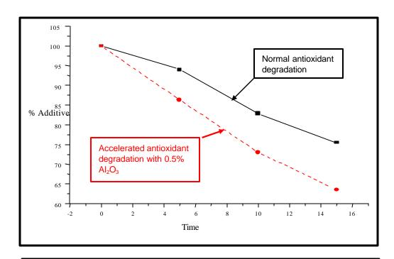
**Fig. 5** Depicts the antioxidant degradation slopes of the SAE 15W40 Engine oil: Red curve: in the presence of  $Al_2O_3$  Black curve: without the presence of  $Al_2O_3$
