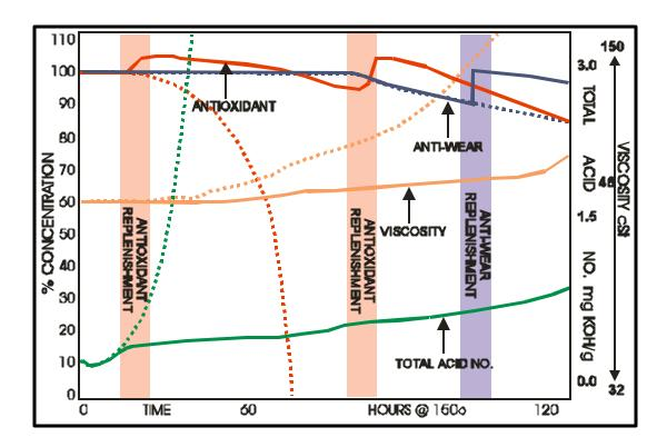
**Fig. 7** Is the same typical fluid degradation graph as Fig 1 except that the antioxidant was replenished at two different intervals and the anti-wear was replenished once. As a result of the first antioxidant replenishment the TAN stabilized and therefore kept the viscosity from increasing. This was repeated a second time as the antioxidant reached its minimal level again.
