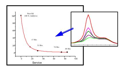
**Fig. 4** Box on the right shows how using FT-IR spectroscopic analysis depicts premature additive degradation due to a chemical reaction with the antioxidant and alumina dust found in an aluminum smelter. This superimposed degradation is then transposed to the curve in the box on the left.
