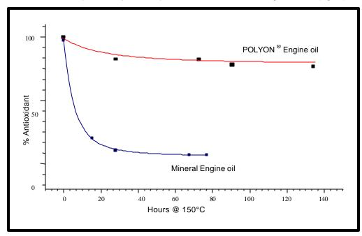
**FIGURE 6:** Comparative antioxidant degradation curves (in the presence of aluminum dust) of semi-synthetic POLYON® vs. the customer's traditional mineral based engine oil.
