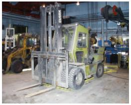
Preliminary tests on mineral-based motor oils traditionally used by the facility showed premature oxidation and increased viscosity. FT-IR analysis showed a quick, distinct reduction in performance additives, particularly the antioxidant (Fig 4 above). The end user reported that the life-span of these fluids *never* surpassed 75 hours of use and that the engines had to be rebuilt every 9 to 12 months!
