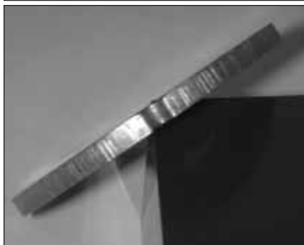
Fig. 7. Scratches visible on the side of the pump plate.
