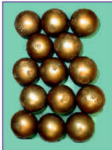
Fig.3 Ball bearings exposed to heat levels beyond their original design. Note how they lost their spherical form and created scuff marks on the surface by due to sliding.
