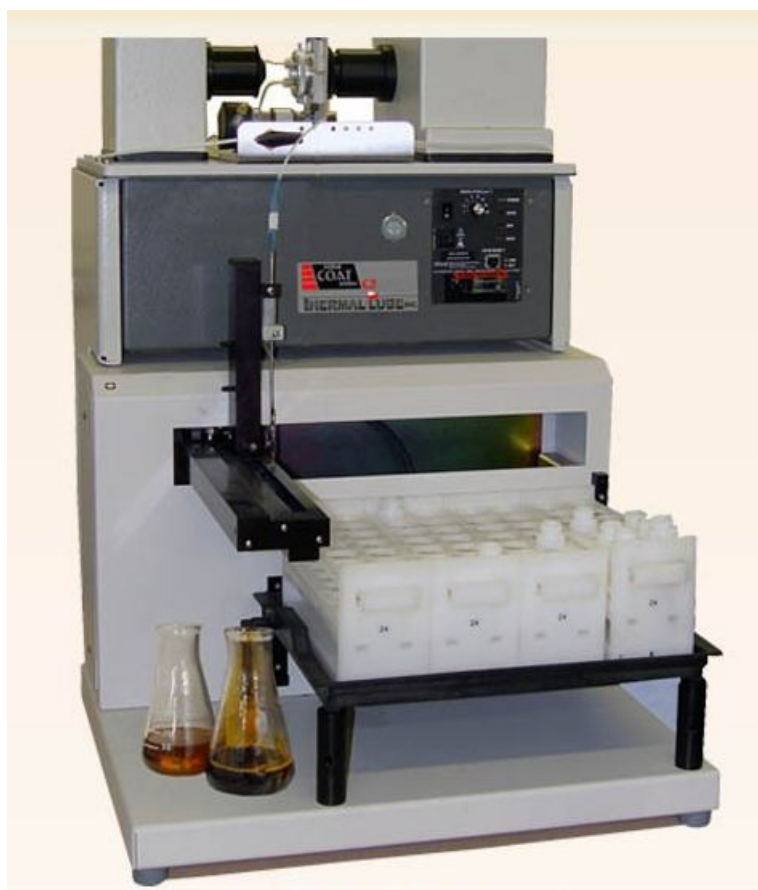
Figure 1. COAT system for the quantitative FTIR analysis of AN, BN, H 2 O.
