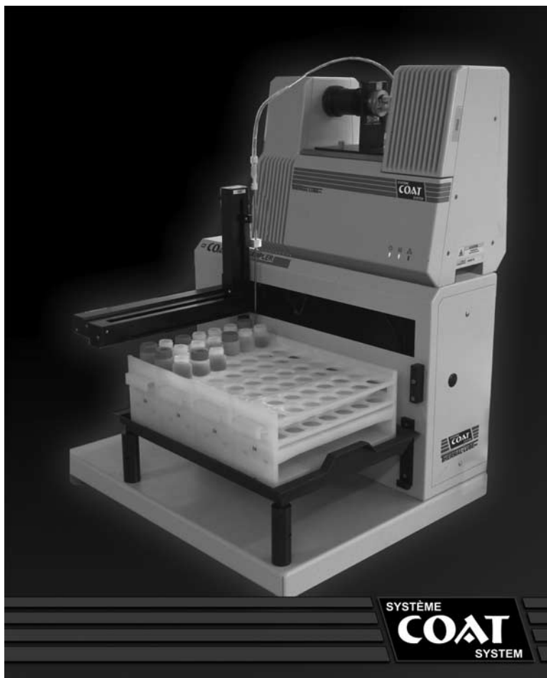
FIG. 3—The COAT system, an integrated auto-sampler and FTIR analyzer designed for lubricant analysis, capable of carrying out qualitative FTIR CM as well as analyzing oils quantitatively for AN, BN, or H_2O at throughput rates of up to 180 samples/h.
