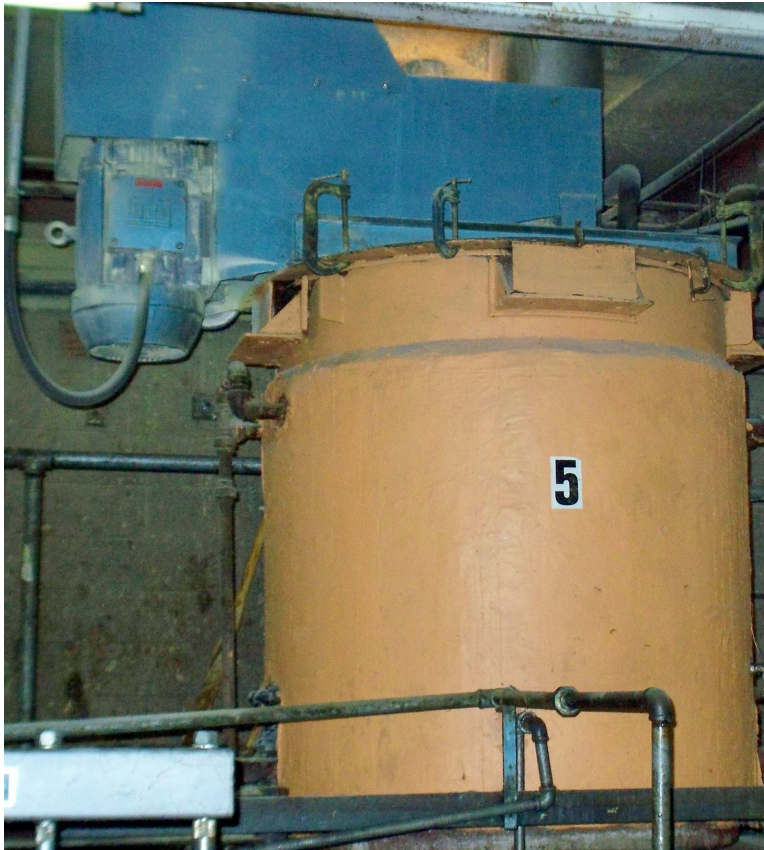
Fig 1. 1500Kg Lubricant Blender. (courtesy Thermal-Lube Inc.)
