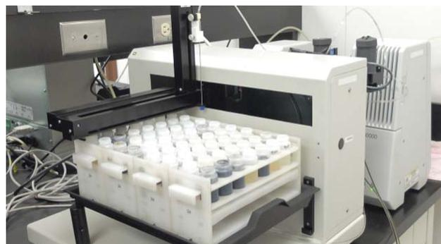
Figure 1. An example of a system used for the FTIR determination of ASTM-identical acid number and base number results for in-service mineral oils
